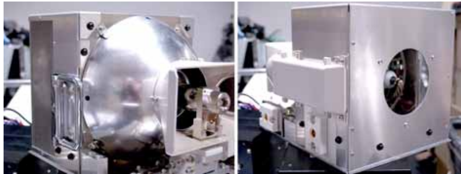
Figure 4 – Remove Lamp Cover-3.0kW
